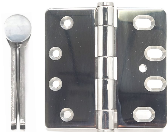
#42.4613; Left Hand (LHR) 304 Polished Stainless Steel Heavy Duty Hinge 4 x 4 x 1/8 inch. Removable Pin. Spacing: 5/16" When Folded Barrel 9/16" diameter
