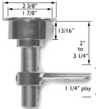
#43.964 Hatch fastener with cam With roller bearing cam: #43.975 Lifting / turning lever #43.974 48 mm diameter; up to 25 mm material thickness, with back plastic counter plate see also page 4-3-1.
