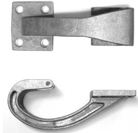
#42.524C - C-Hinge Bracket 7"x 17.5" Max weight hatch: 300 lbs. Parts casted aluminum alloy not painted.
