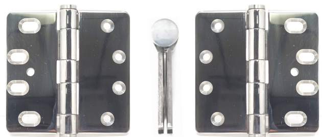
#424611 Metric LHR #42.4612 Metric RHR Size: 100 x 100 x 3.2mm. Distance when folded 8 mm Barrel: 14 mm diameter 304 Polished Stainless Steel Heavy Duty Hinge
