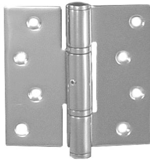
#42.236 Hinge 90 x 100 x 3 mm Pin: 16 mm Pin has set screw, cannot be removed 3 1/2" x 4" x 1/8"
