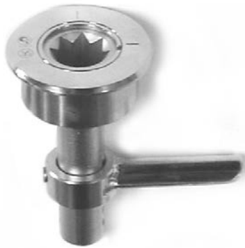
#43.964 Hatch fastener with cam With roller bearing cam: #43.975 Lifting / turning lever #43.974 48 mm diameter; up to 25 mm material thickness, with back plastic counter plate see also page 4-3-1.
