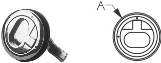
Hatch fastener #43.1954 (set) Includes: Cam and strike. Dimension A = 3 1/2" diameter Dimension B = 3 3/4" Cut hole 3" diameter Standard spring loaded strike included.
