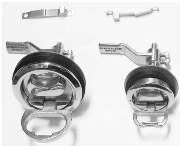
Hatch fastener #43.1954 (set) Includes: Cam and strike. Dimension A = 3 1/2" diameter Dimension B = 3 3/4" Cut hole 3" diameter Standard spring loaded strike included.
