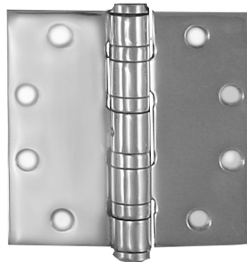
#42.1150 Hinge 4.5" x 4.5" x 3/16" with stainless steel ball bearings 316 stainless steel.
