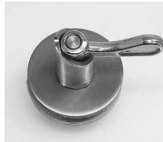
#47.281 Spring Loaded Indexing Plunger threaded M20' x 1.5 Shown with 50 mm diameter threaded thrust roses #15.050 through 10 mm Acrylic. Stainless steel; throw: 5/8"; body diameter: 3/4" Body length: 3"; threaded M20 x 1.5
