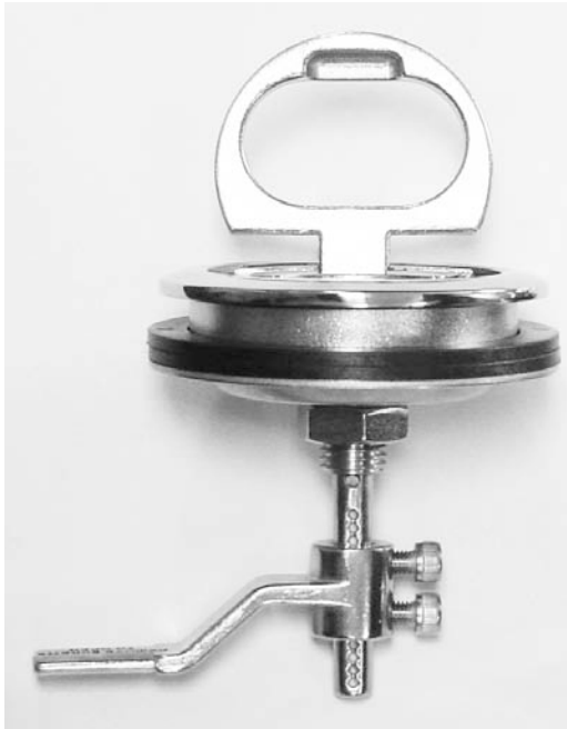
#43.1954 hatch cam lock with lift ring Diameter 3 1/2" Cut hole 3" + Distance Cam from body: 3 3/32 inch to 1 inch Minimum hatch thickness: 5/16 inch
